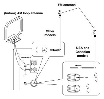
Strip away the insulation from the end of the cable, then fully insert the stripped end of the cable.
